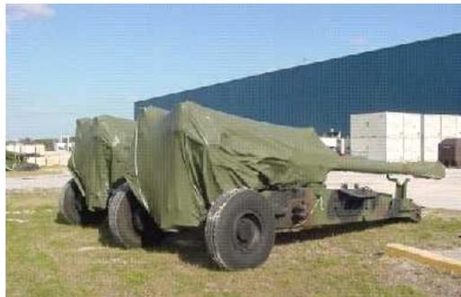
**Figure 1:** Image from Transshield commercial literature illustrating cover on the body of a howitzer. (Transshield, *The Shrinkable Fabric* (2006) [www.transshield-usa.com/military.html](http://www.transshield-usa.com/military.html))
